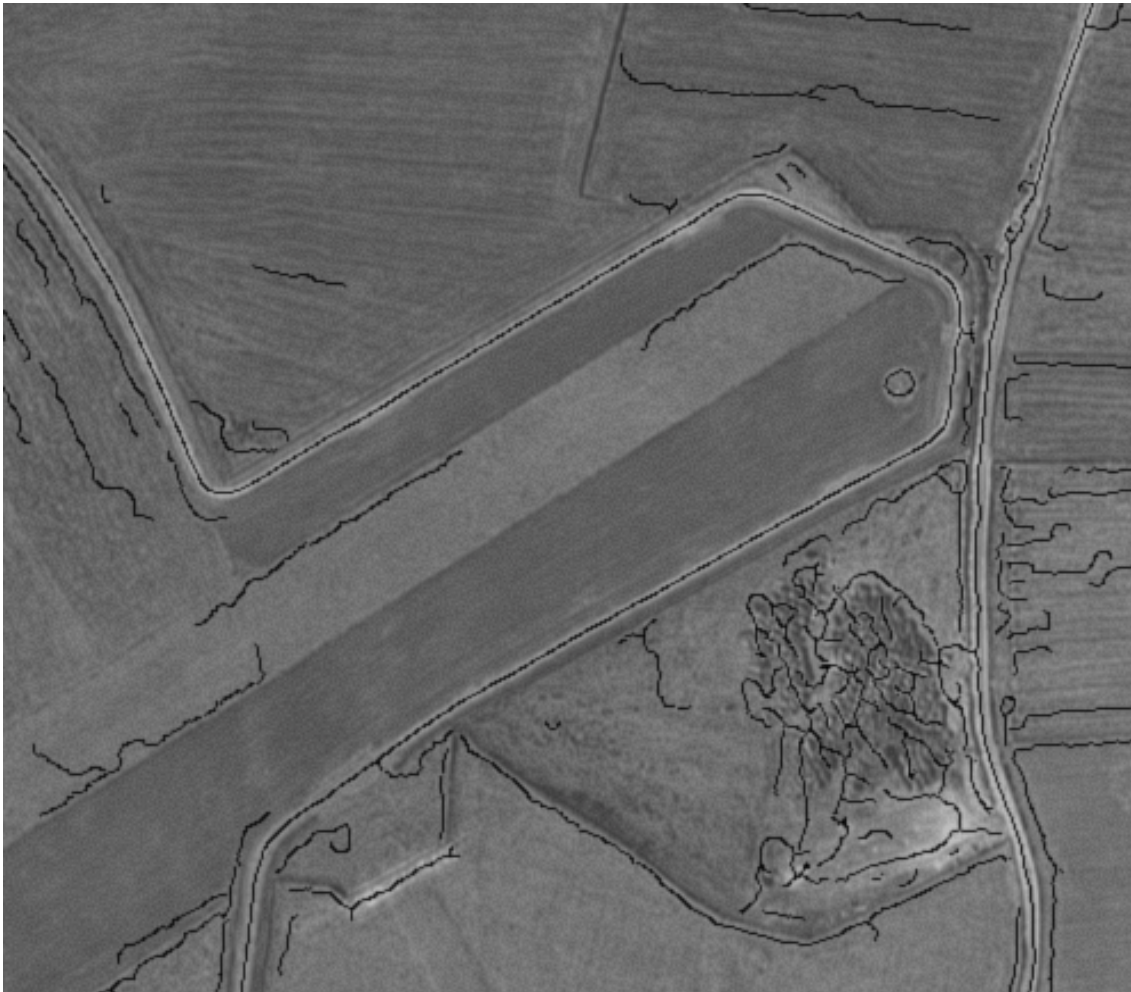
Figure 4-28: Output of the “Steger Line Detector” Algorithm.
