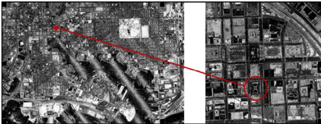
Figure 4-2: Requirement of Multi-Scale Localization. A rendering of a portion of a Baltimore LIDAR data set as an image (left) with a zoomed view in the vicinity of the domed building (right).
