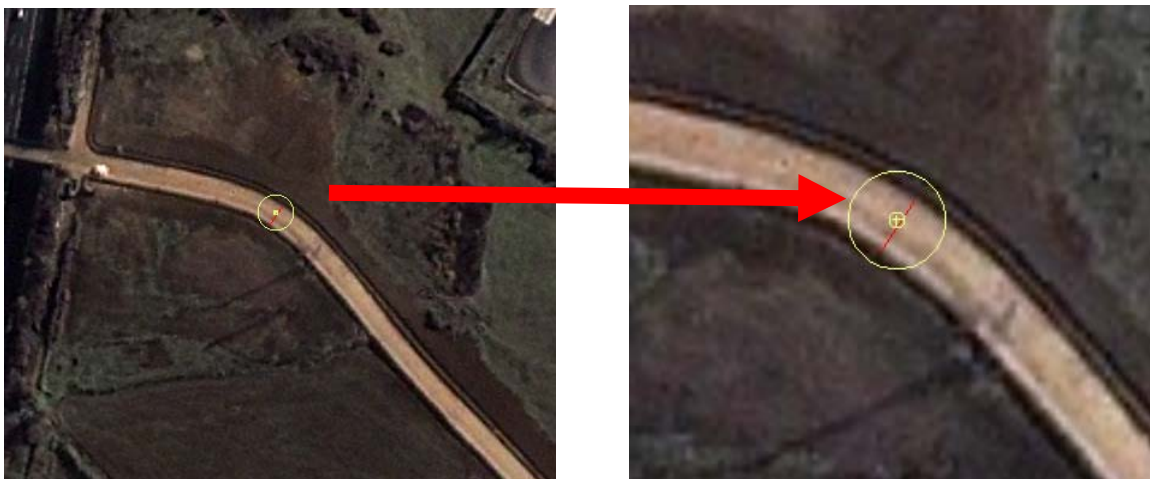
Figure 4-27: Boundary Detection – the Roads to Extract (left) and the Detected Boundaries (right).
